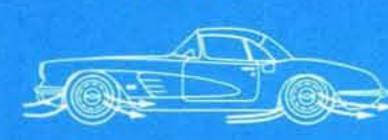
New Radius Rods Improve Performance! New rear suspension, with radius rod rear axle control, is an outstanding engineering refinement in the Corvette. Radius rods relieve rear springs from axle housing torque reactions during acceleration and braking, thus improving performance and stability through a smoother flow of power. Rear axle steering movements are free of the torque influence, giving consistent handling precision.
